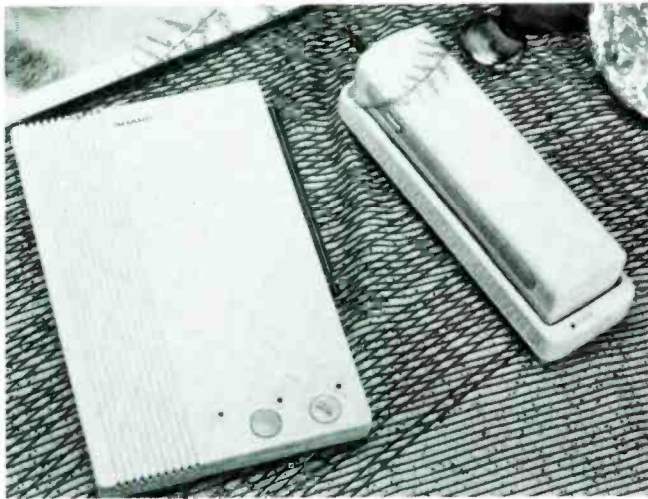
Sharp's CL-300 is a stylish cordless phone that can also function as an intercom. The base unit can function as a speakerphone, and a regular telephone can be plugged into it for normal conversations when the hand unit is elsewhere.
