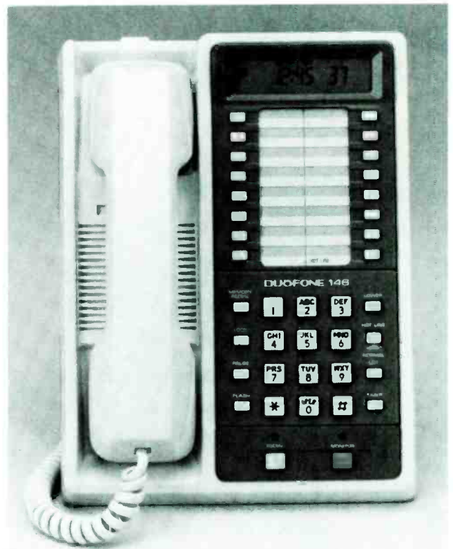
Radio Shack's DuoFone 146 features a 32-number memory, demon dialing, a call timer, and a hot-line dialer. When using the hotline dialer a stored number is dialed automatically whenever the receiver is lifted.
