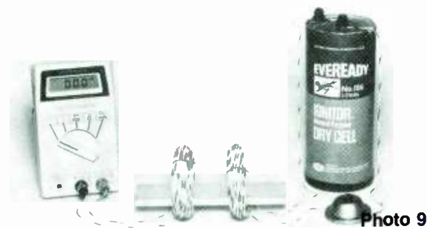
Shown here is the apparatus for recreating Michael Faraday's discovery of electromagnetic induction. A couple of banana plugs are used to connect the coil to the voltmeter.
