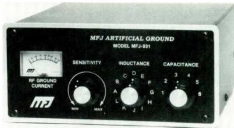
The Model MFJ-931 artificial RF ground (pictured here) is series connected in the antenna ground return line and is used to tune the ground wire.
